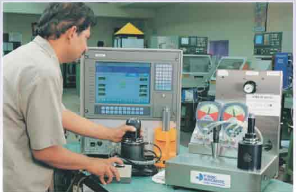
▲ AT3 TAPER CHECK ON AIR ELECTRONIC GAUGE
