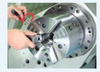
2.Turn T-handle clockwise to tighten and the jaw is locked.
