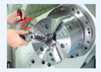
1.Turn T-handle counter clockwise to release and move jaw forward to its position.
